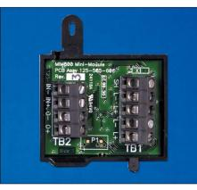
The MIM800 is a small MX addressable module designed for monitoring a single input circuit. The MIM800 can monitor normally open or normally closed inputs and provides open and short circuit monitoring of the line
