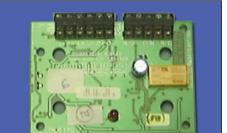
The RIM800 provides a single programmable relay output from the MX DIGITAL addressable loop which can be programmed for a variety of applications including signalling fire conditions to plant, machinery, fire doors, dampers & security systems. The RIM800 relay coil is monitored. The RIM800 relay contact is rated for 2A @ 24V d.c. but can be used to switch mains voltage when used with the HVR800.
