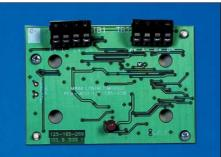
DIM800 Detector Input Module
